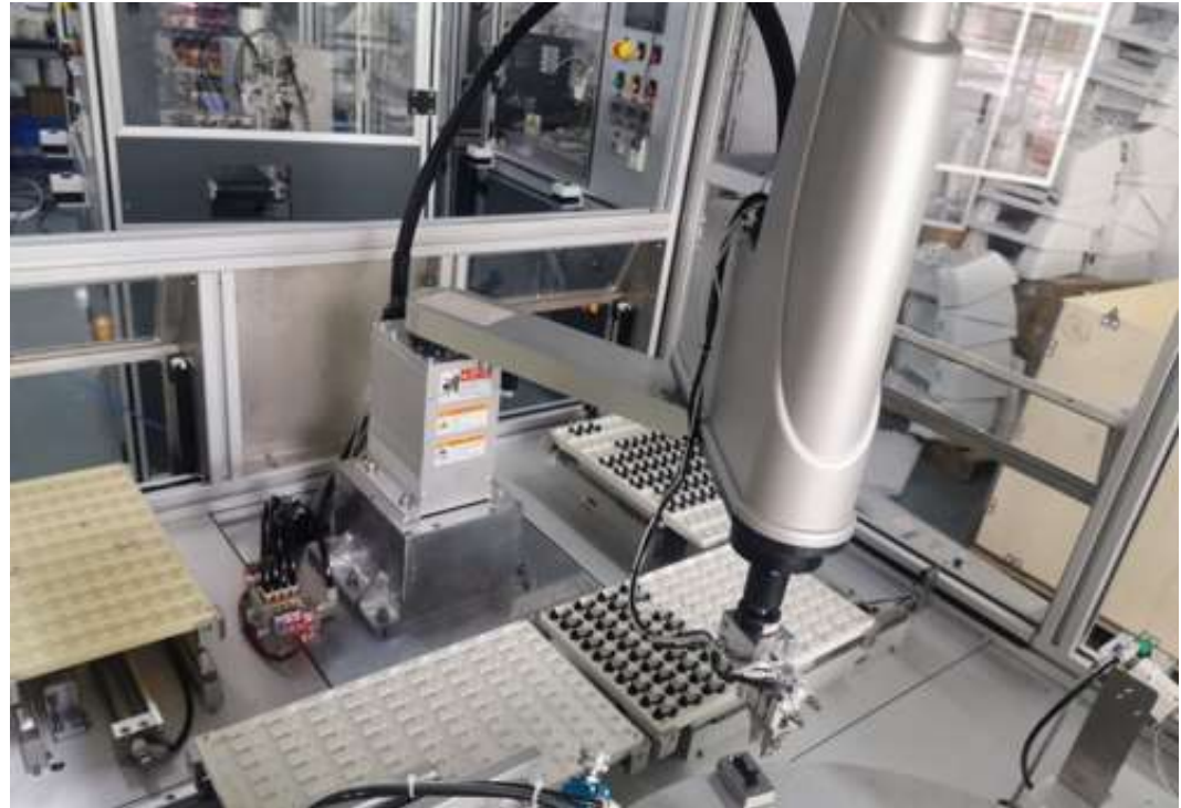
Robot Arm and Vision Inspection System
